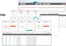
A Virtual Packet Broker (vPB) works just like a physical Network Packet Broker, as a scaled-down version that can run on a standard hypervisor in the virtualized data center or the cloud. It can aggregate, filter, and process the network traffic between the virtual machines (VM) in the east-west direction, and forward to the tools for monitoring and analysis, which is otherwise a major blind spot.
